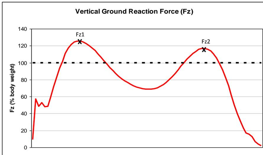
Figure 1: Graph of Fz for a healthy adult during one stance phase, showing both peaks (Fz1 and Fz2) greater than 100% body weight
