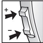
When volume is increased or decreased, a beep signal will be heard for each incremental change. When the upper or lower limits of the volume range are reached, the beep will change tone. During the fitting of your hearing device, your hearing care professional will have chosen an optimal volume setting for you. When switching the hearing device on, the volume will have this optimal setting.
