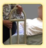
NON-compliant: If gaps are larger than 120mm in both a vertical AND horizontal direction as this could cause a head or neck entrapment. – the vertical gap should be measured from compressed mattress height
