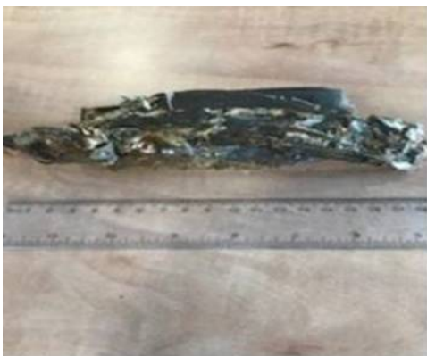
Figure 1: Metal piece that caused damage and delay in clinical waste treatment facility.
