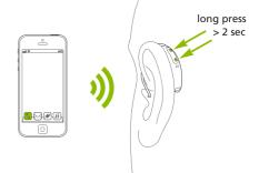
An incoming call can be rejected by a long press on the upper or lower part of the multi-function button
